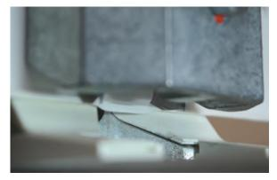
turn over the profile on the head - put it straight on the trestle - lock the clamping device - cut very carefully
